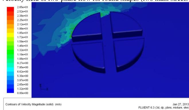
Figure 7: contours of Velocity field of two-phase flow for round shapes (2 main streets and  $\Theta=30^\circ$ )
