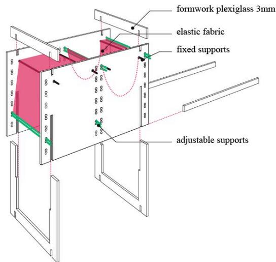
**Figure 3.** Free hanging fabric formwork set up.
