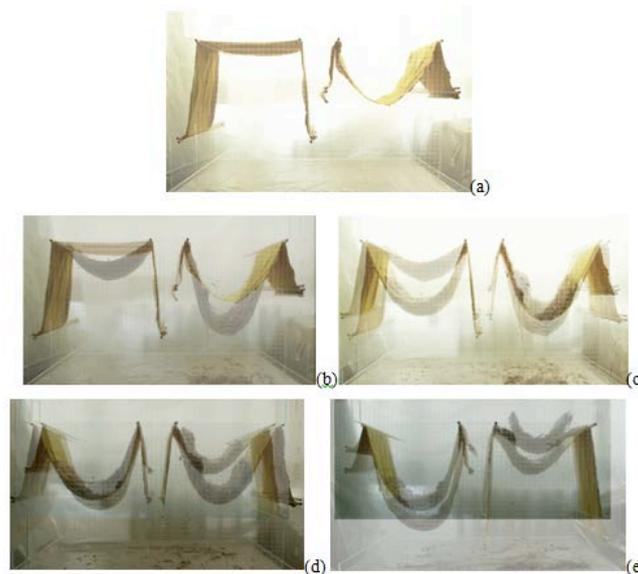
*Figure 4.* Form finding situations in five phase: (a) initial phase of free hanging fabrics, (b) superposition of initial phase and first phase –form after loading MbM, (c) superposition of second phase and first phase, (d) superposition of third phase and second phase, (e) superposition of third phase and fourth phase.
