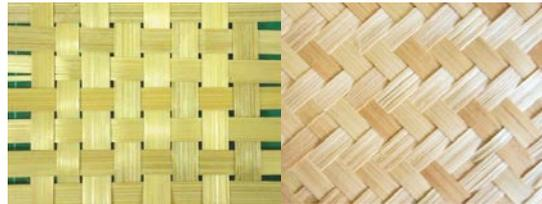
*Figure 5.* Single and double pattern of biaxial woven patterns.
