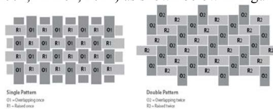
Figure 1. Two Dimensional of Traditional Weaving Configuration.
