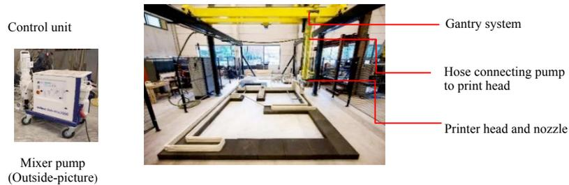
Figure 1. 3D printing facility at TU/e, with some examples of printed objects.
