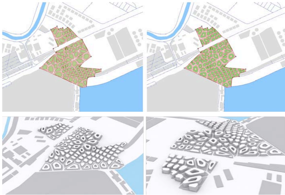
Figure 5. External Geometrical Setting to Voronoi Tessellations (Top Left), Creation of Internal Polygonal Spacing (Top Right), Proposal 3D External Shots (Down)
