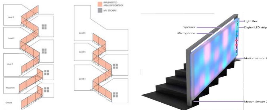
Figure 5. Section of Application Areas and Light Box Design
