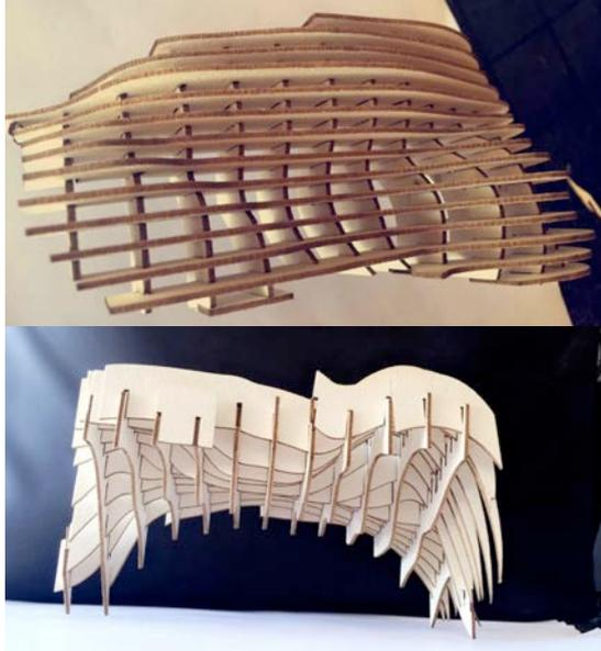
Figure 1. 1<sup>st</sup> group prototype using the system of waffle structuring
