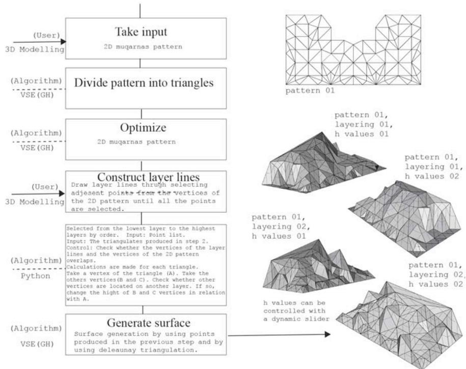
Figure 8. Algorithm schema of the 3D form generation process and samples of 3D surface geometries produced from the same 2D pattern but different layering method.
