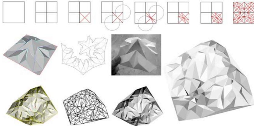
*Figure 7.* Mapping 2D pattern onto 3D surface.
