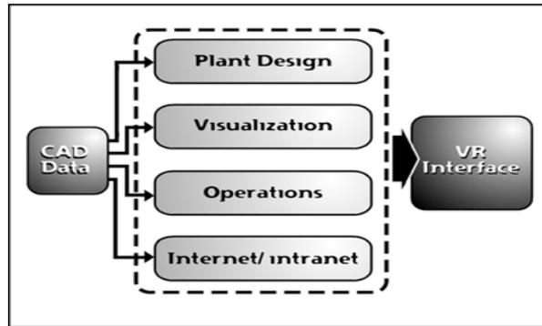
Figure 2. A conceptual diagram showing how CAD data can be combined with other content information to form an integrated VR interface design.
