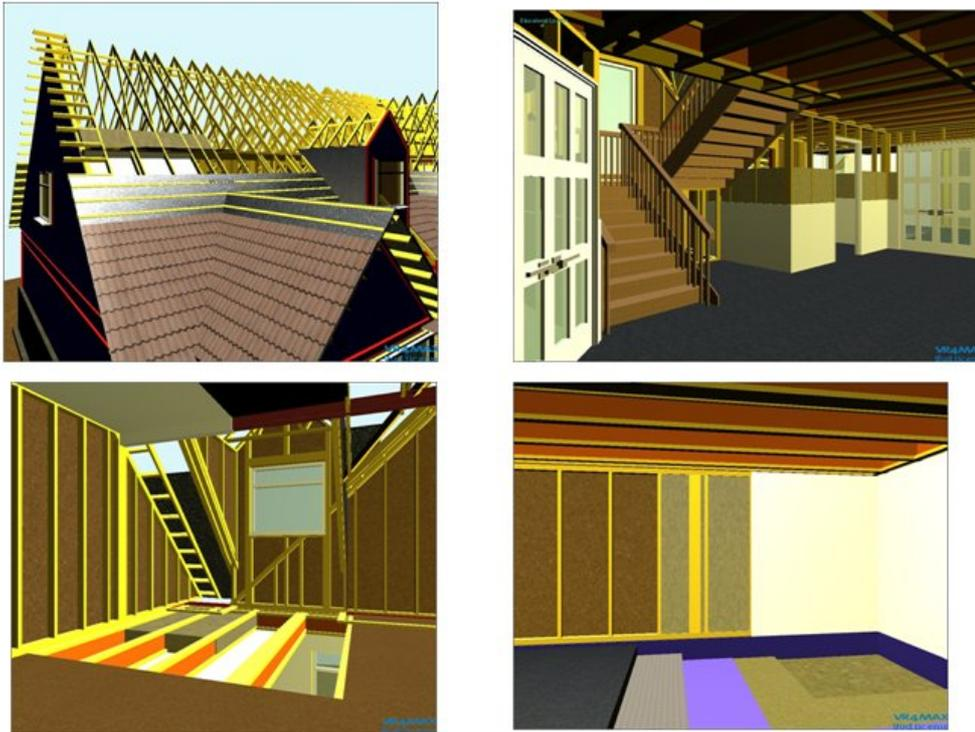
Figure 4. Fully interactive VR model of timber frame house showing construction details.
