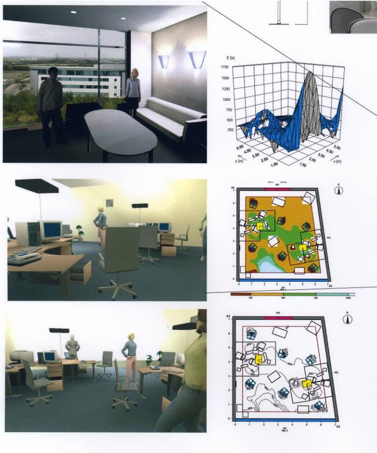
Figure 5. Lighting studies detailing the factors contributing to good lighting design for a successfully serviced media centre (Student: Edward Miley).
