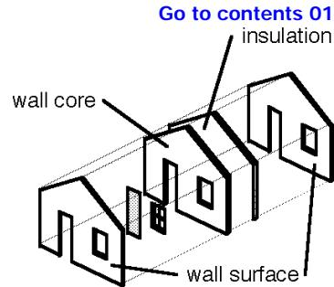
Figure 5 (right). Core wall construction
