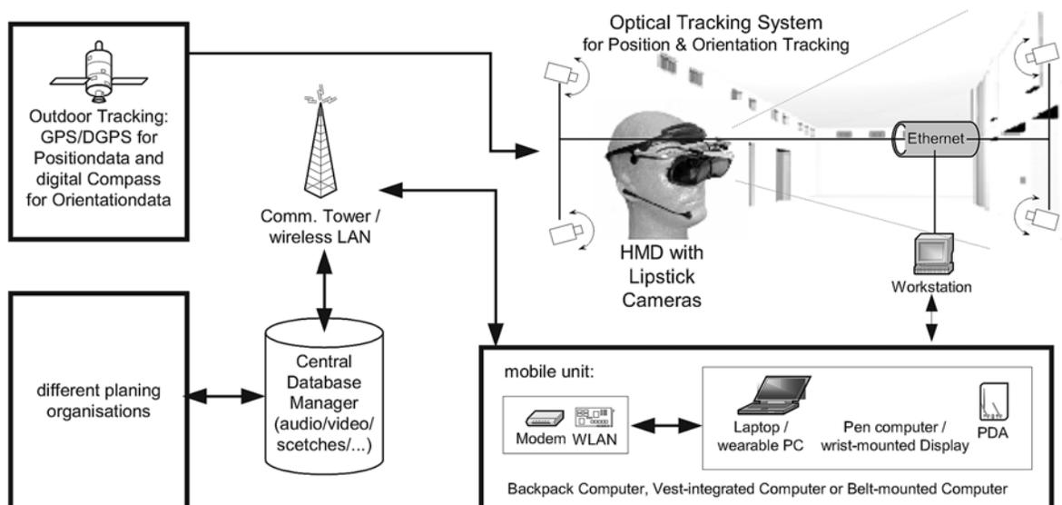
*Figure2. The concept of an current system architecture.*
