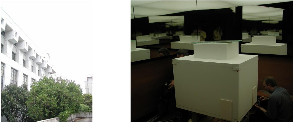
**Figure 1.** Artificial skies enable building designers to quickly simulate for a variety of conditions that may be difficult to control for in the real world. (left) an actual building under overcast skies and (right) a physical model in a calibrated chamber
