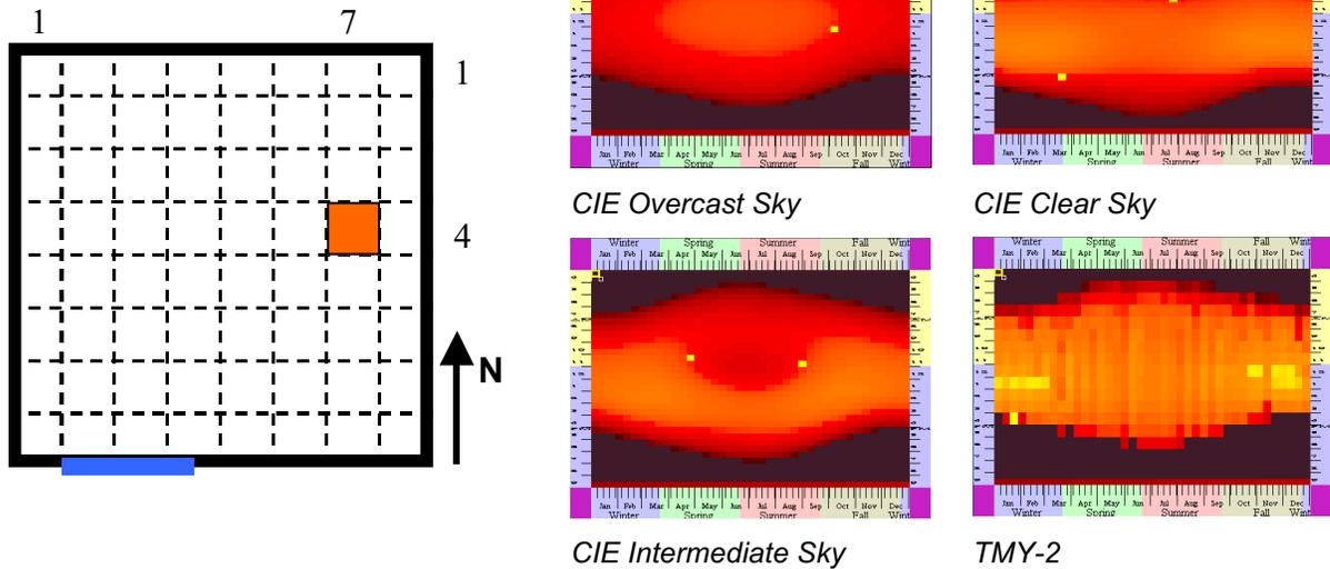
**Figure 4.** (left) A rectangular model with a single South-facing window. (right) The performance under four sky conditions across the year.
