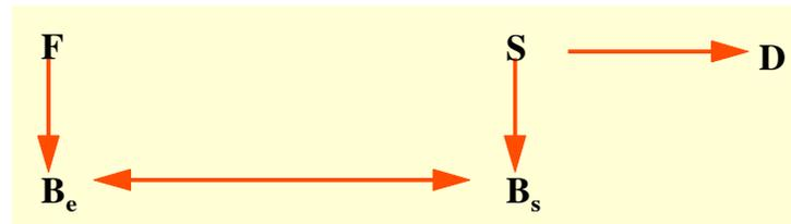
Fig. 2. The F-B-S model, where the behaviour is bifurcated into expected behaviour,  $B_e$ , and behaviour derived from structure or actual behaviour,  $B_s$ ; D represents the documentation, ie the formal output of designing;  $\square$  = transformation and  $\square$  = comparison.
