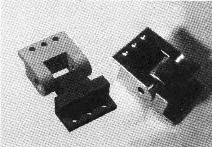
Figure 6. An aluminium hinge and the associated form•Z model.
