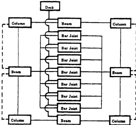
Figure 6. Component network of steel frame building.
