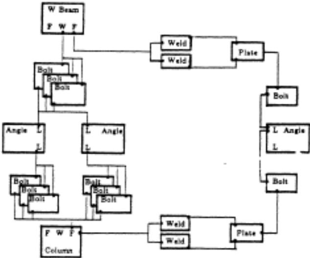
Figure 8. Detailed component network.
