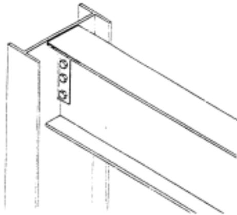
**Figure 1. Shear tab beam to column connection.**
