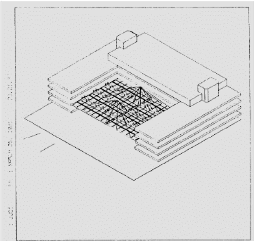
Fig.1 Pen plot of tension assisted structure produced from CATIA (courtesy M.K. Rodwell).
