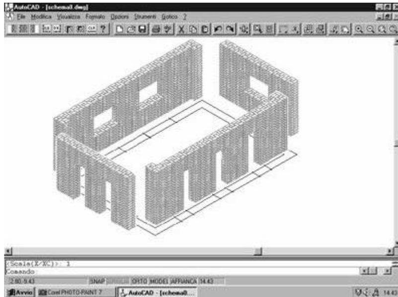
**Figure 8. The complete external wall: exploded view. In this phase the general consistency control of opposite walls is made.**
