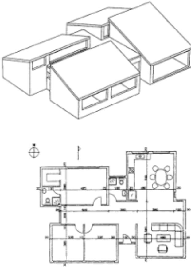
**Figure 12.** A perspective view and documentation of the passive solar building. The geometrical data base, needed for the 3D model and the 2D drafting system, was automatically built by the knowledge based system.
