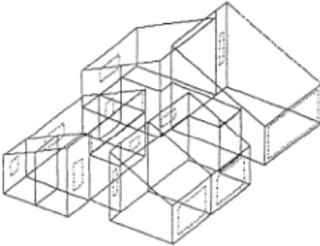
**Figure 7.** An axonometric view of the proposed building with the recommended area for each window (alternative # 1). The system locates the windows in the middle of each wall.
