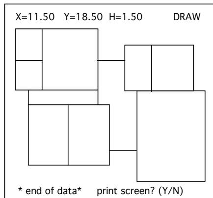
**Figure 5.** The introduction of the building geometry by a schematic plan (using the mouse) and heights at each corner (using the keyboard).
