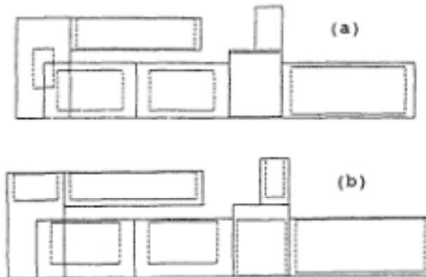
**Figure 8. a.** The windows on Southern elevation as proposed by the system. The designer can now change the locations of windows very easily. **b.** The windows on Southern elevation as were changed by the designer.
