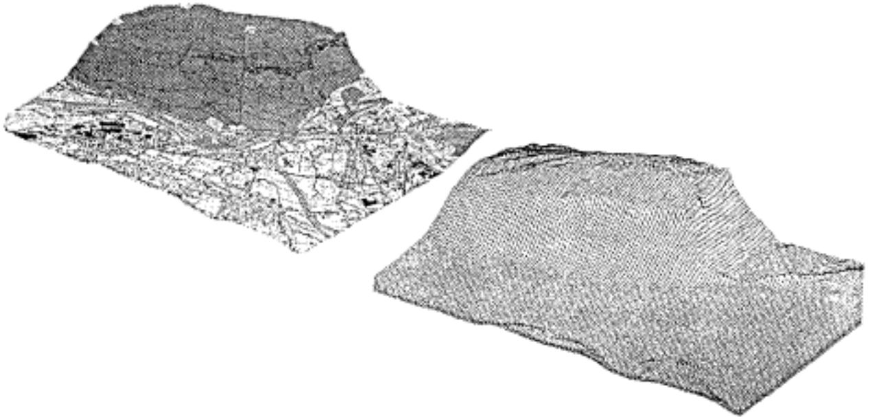
Oltén (2): Digital topography model (DTM) with pixel map draped over it and as mesh representation
