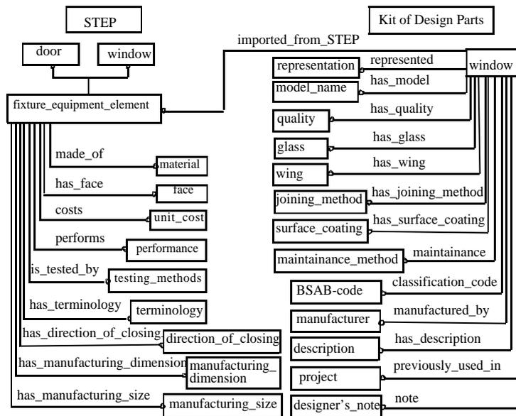
*Figure 2.* Illustration of information about windows that may be stored in the model of design parts.
