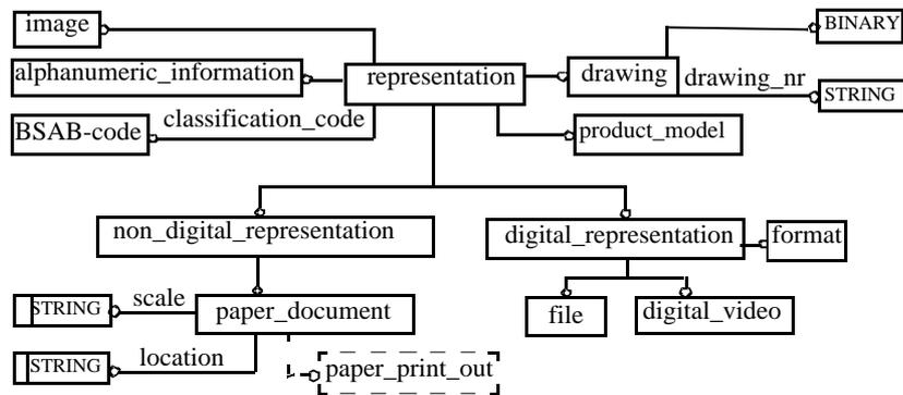
Figure 3. Basic structure of the representation object.
