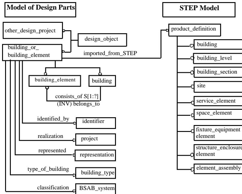
Figure 1. Basic structure of the model of design parts.
