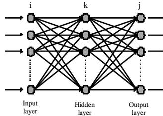
Figure 1. A typical multi-layered back propagation network.
