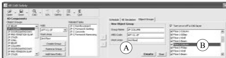
Figure 7. Grouping Function (A) and Turning On/Off Layer Function (B)
