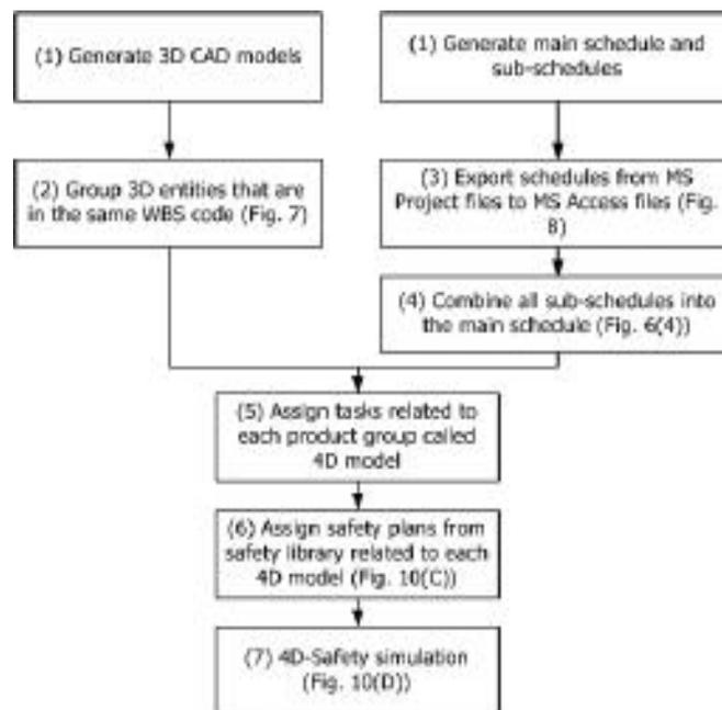
Figure 9. Flowchart for Generating of 4D-Safety Simulation
