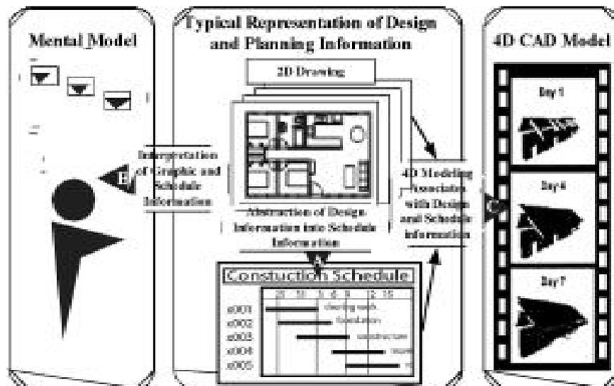
Figure 1. Comparison of Traditional Representation of Construction Information and 4D model (Source: Modified from McKinney, 1998)
