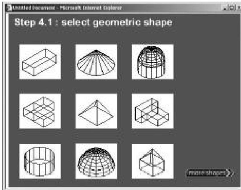
Figure 4 . Select Geometric Shapes from the Standard Shape List
