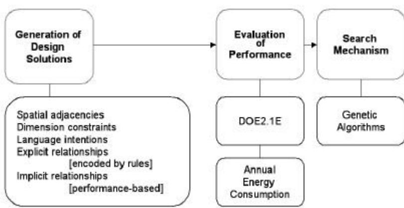
Figure 2. Flow chart of the Generative Design System presented
