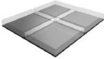
*Figure 4.* Graphical representation of 1<sup>st</sup> floor room constraints. Each room could have at most 15 x 15 m, with minimum dimensions of 3m.
