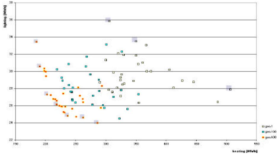
Figure 9. Progression of Pareto front search, from generation 1 to 400. The shaded squares indicate points visualized in figures 11 and 12.
