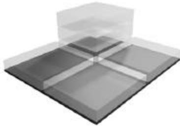
*Figure 5.* Graphical representation of 2<sup>nd</sup> floor room constraints. Space height can vary between 3 and 6 m. The topmost volume indicates maximum roof height.
