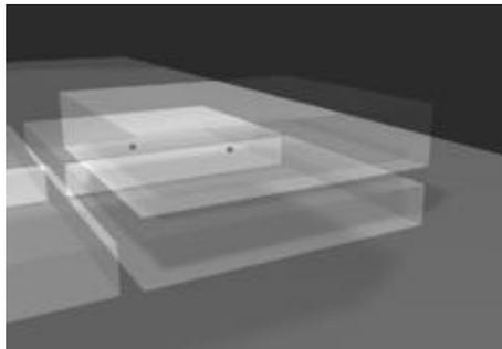
*Figure 6.* The two dark dots represent daylighting sensors automatically placed by the GA inside a 2<sup>nd</sup> floor room
