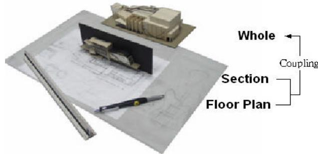
Figure 2. The designer organizes information by coupling a physical section model with the floor plan in a spatial setting.
