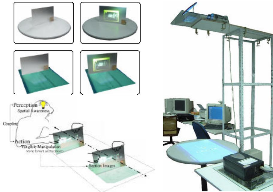
Figure 3. The setup of the interactive table
