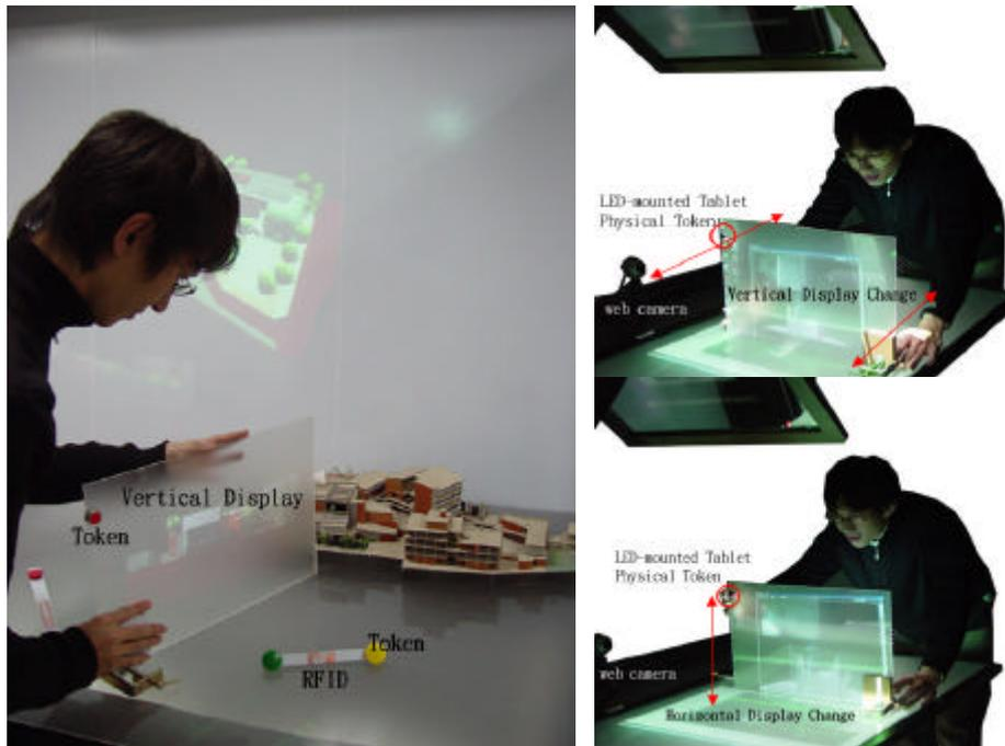
Figure 7. The prototype consists of horizontal display and vertical display for representing 3D geometry interactively through placing LED-mounted tablet and manipulating physical tokens.
