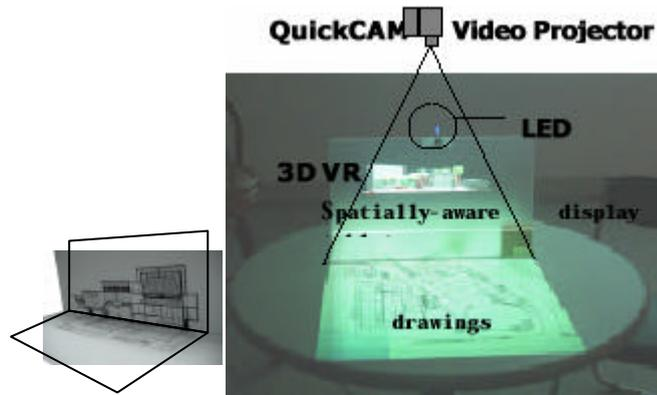
Figure 4. A semi-transparent tablet can be dynamically placed on the plan drawing to display spatially-contiguous section images of a 3D digital model.
