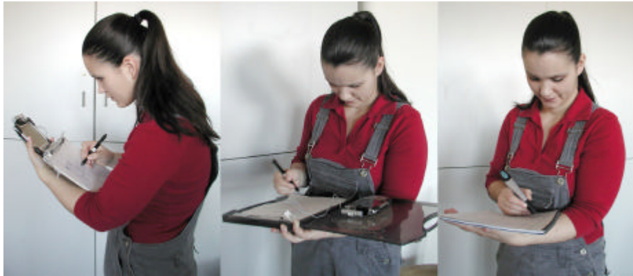
Figure 2. Some tools are easier to use than others. At left, the Inklink connects to the iPaq with a tiny cable and to a notepad with a clip, all hard to hold while sketching. By using a plastic file folder to hold the tools, center, the devices are slightly easier to use. On the right, the standalone Iopad pen can be used like a normal pen with a special notepad.
