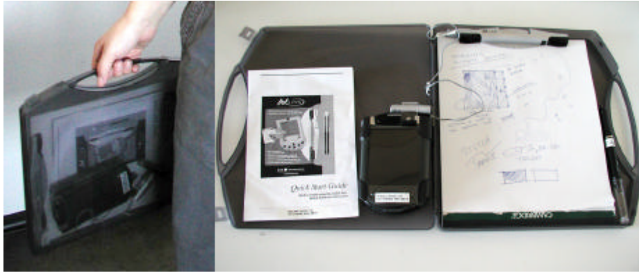
Figure 3. Details of the plastic file folder we improvised for using the Inklink.
