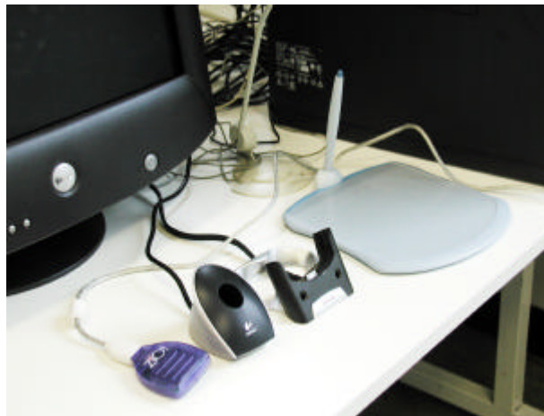
Figure 4. Cradles for transferring information lead to traffic jams at the computer. From the left: Zio memory card reader, Io Pen cradle, iPaq PDA cradle, and Wacom mouse tablet.
