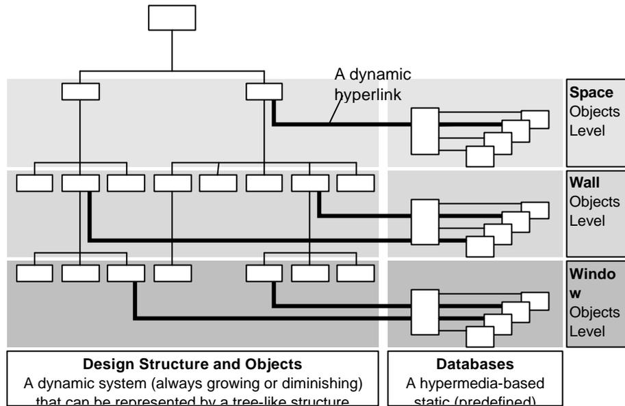
Figure 1. The design creation module automatically builds hyperlinks from the dynamic design structure to specific locations of construction databases when a new object is created.
