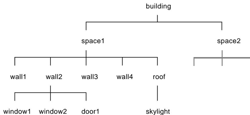
Figure 1. Class hierarchy of building components.
