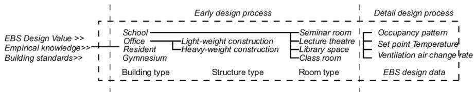
Figure 6. Automating default values of EBS data with database of recommendations and building standards.
