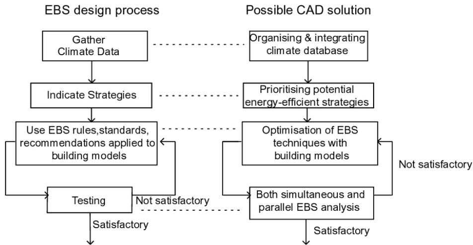
Figure 2. The requirements of CAD functionality in an EBS design process.
