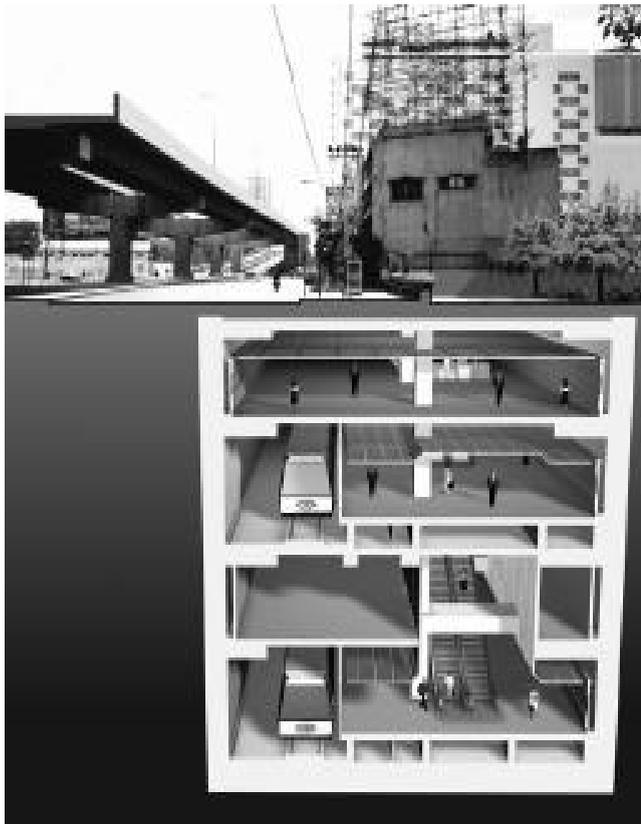
*Figure 5. Stacked platform station in the MRTA project*
