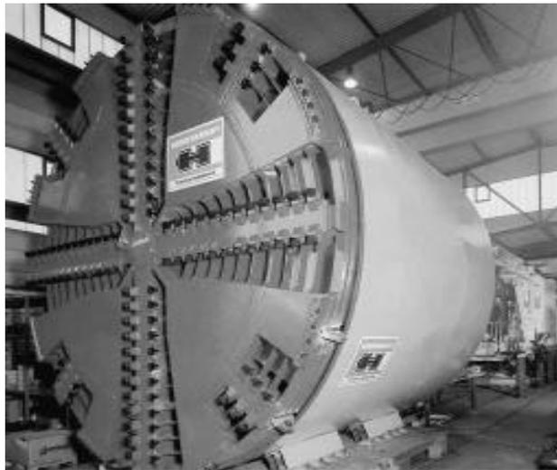
Figure 8. Earth Pressure Balance Shield used in the MRTA project
