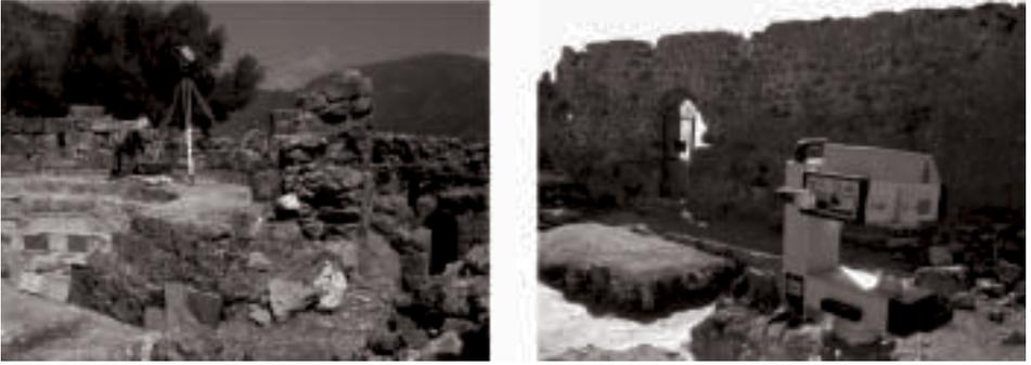
Figure 1. Scanning ruins with a 3D scanner.
