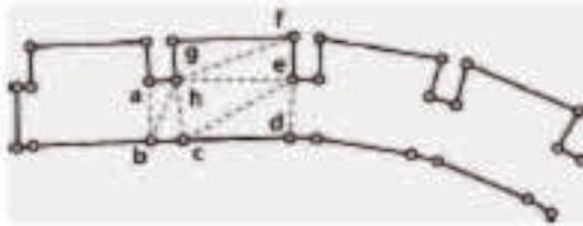
Figure 4. Flattening pattern based on triangular strips.
