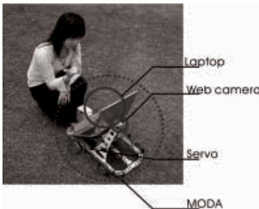
*Figure 4. Hardware components of MODA.*
