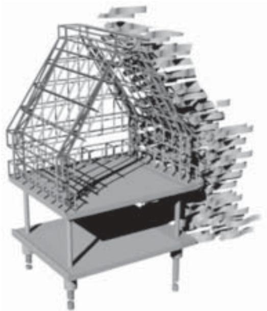
*Figure 4.* Computer section model indicating wind load transfer through primary structure. Phase one. River and Rowing Museum. Henley.
