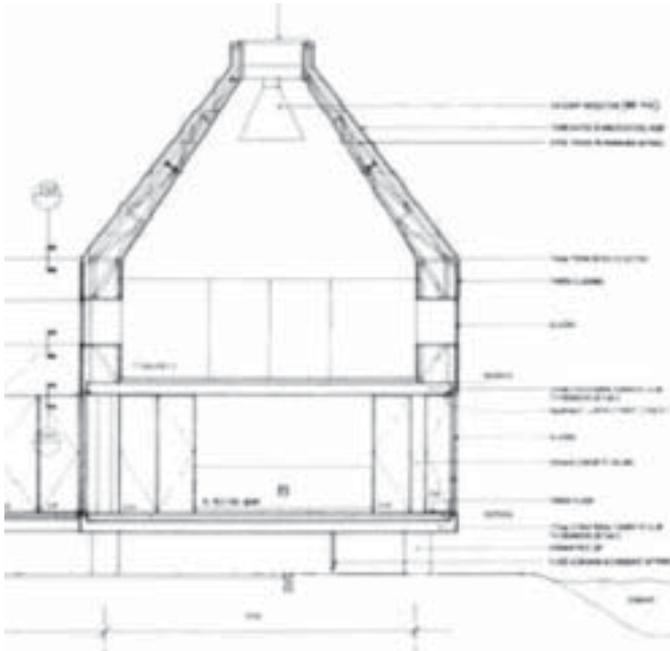
Figure 2. Part general arrangement section through ground and first floor exhibition galleries. Phase one. River and Rowing Museum. Henley. © David Chipperfield Architects.
