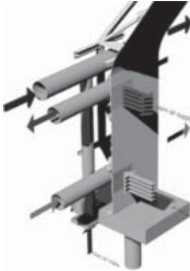
Figure 5. Computer cut away study model indicating air conditioning system integration. Phase one. River and Rowing Museum. Henley.
