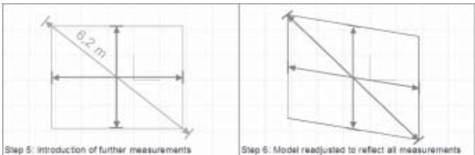
Figure 4. Step-by-step capture of the geometry of a rectangular floor plan, part 3.
