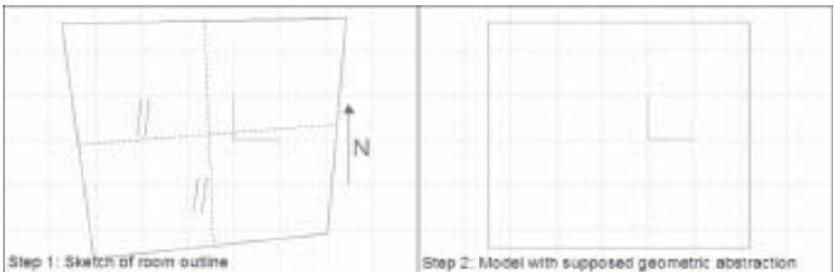
Figure 2. Step-by-step capture of the geometry of a rectangular floor plan, part 1.
