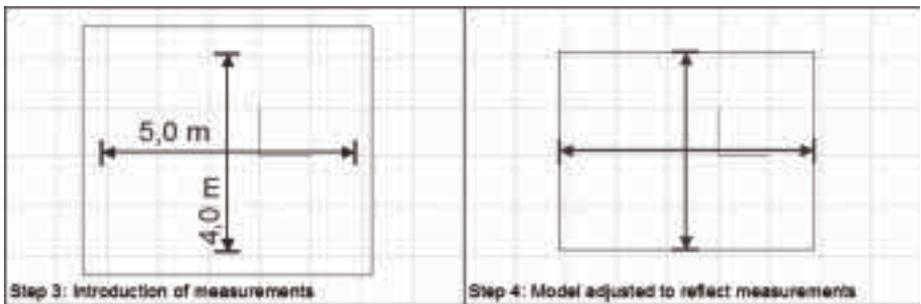
Figure 3. Step-by-step capture of the geometry of a rectangular floor plan, part 2.
