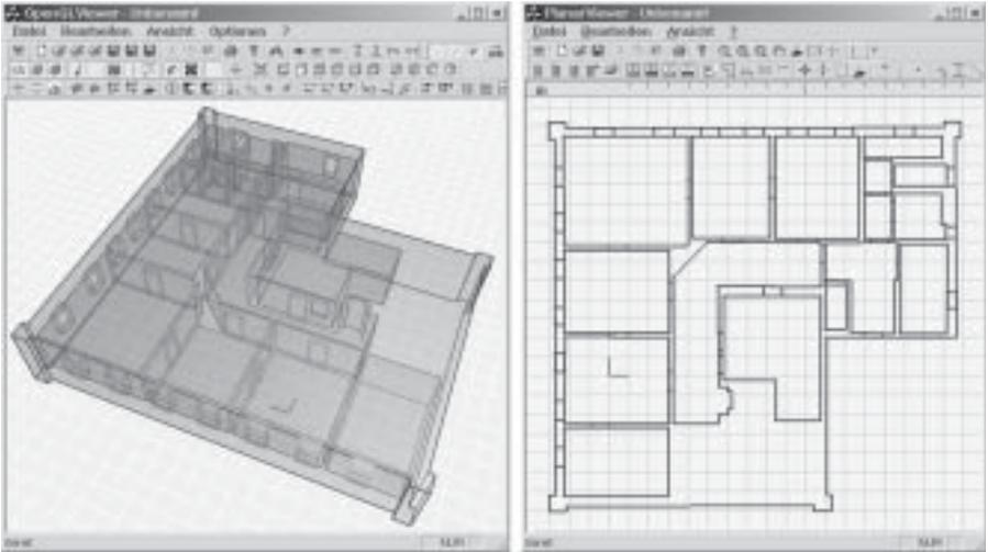
Figure 5. 3D and plan-oriented views of a geometry model using the tools “OpenGLviewer” and “PlanarViewer”, showing an example of a manually measured survey of an office building.
