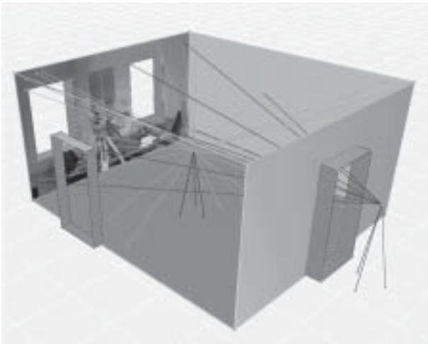
Figure 6. Integrated adjustment : A room containing measurements obtained through manual measuring, tacheometry, photogrammetry and geometric constraints.
