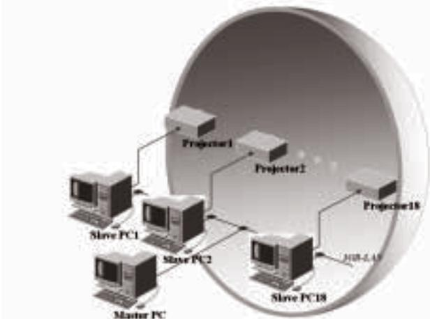
Figure 4. System configuration: A cluster of PCs in master-slave architecture and projectors.
