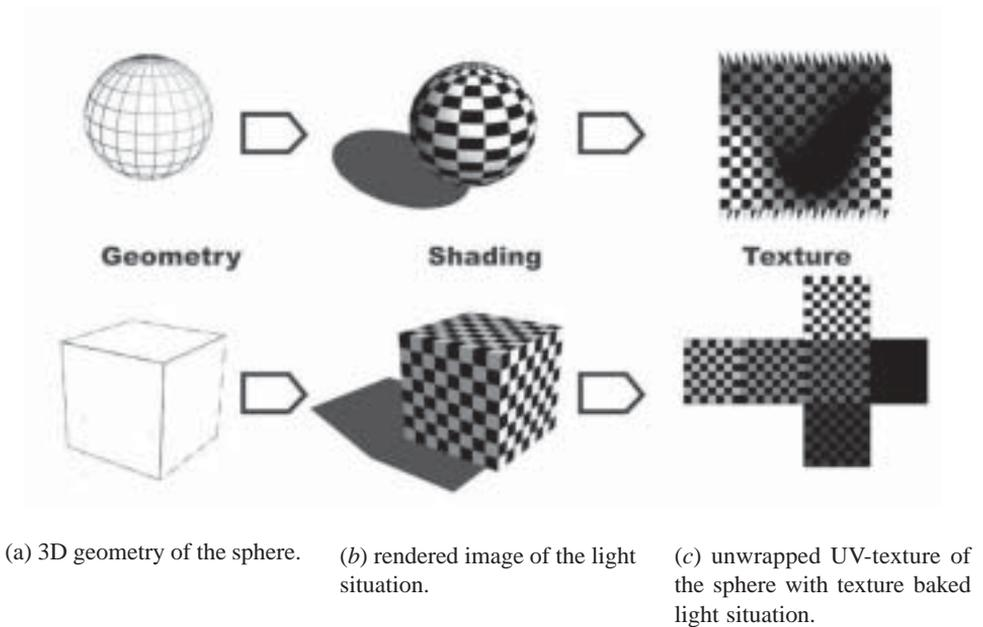
Figure 5. Standard primitives in a simple 3D-scene and their unwrapped texture.
