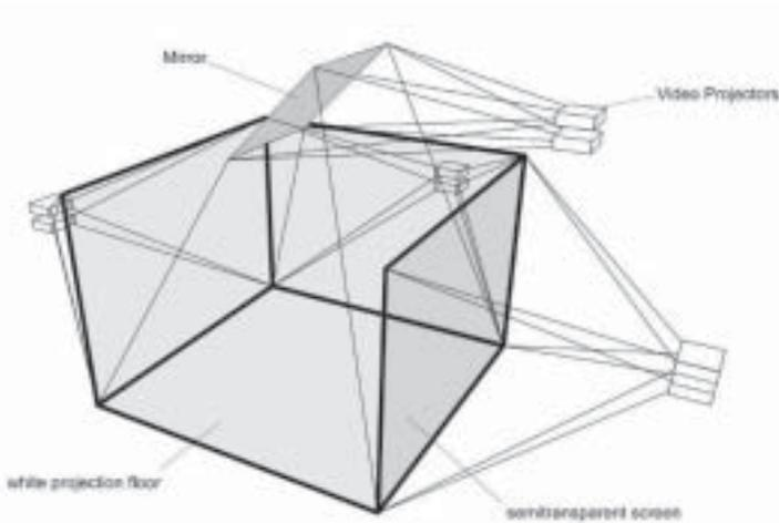
Figure 2. Principle setup of the DAVE at Institute for computer graphics TU Braunschweig / Germany.
