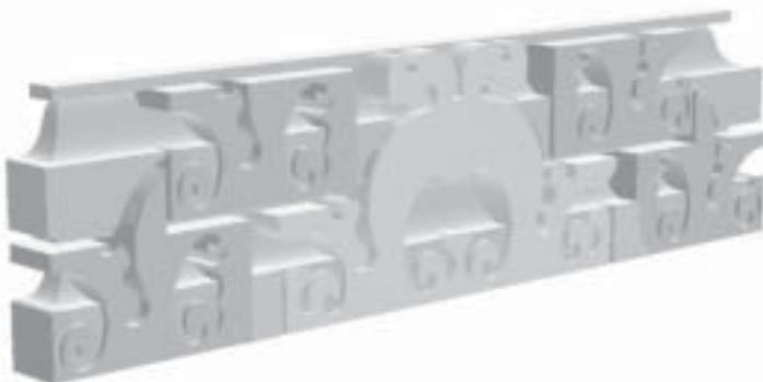
*Figure 3.* Parameterised model of surface geometry of the superstructure. The recovered tile geometry is then combined into a single model. This forms the basis for the repetitive tiling of the surface using a scaling function based on the curve profile shown in Figure 1.
