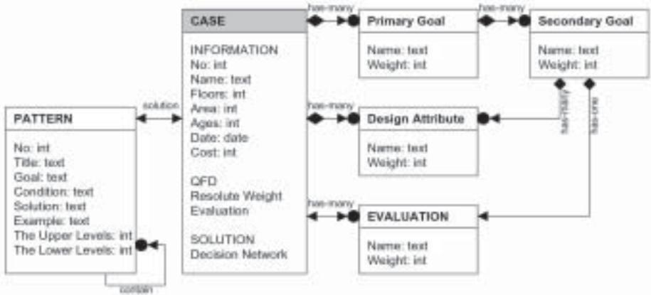
Figure 3. Context diagram of object model.
