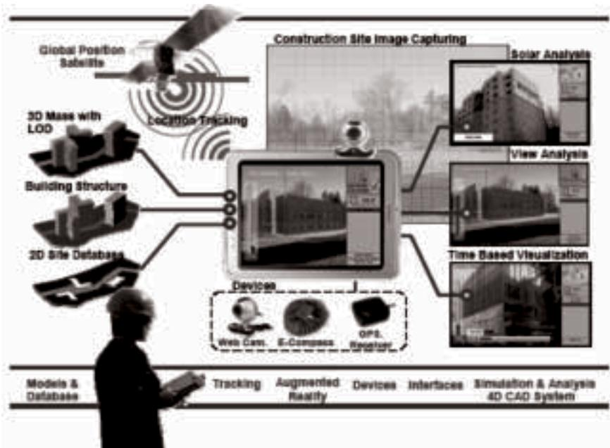
Figure 2. The System Architecture of C-Navi.
