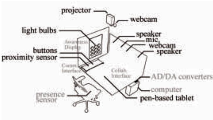
Figure 2. The schematic diagram of our prototype system and its embedded components.
