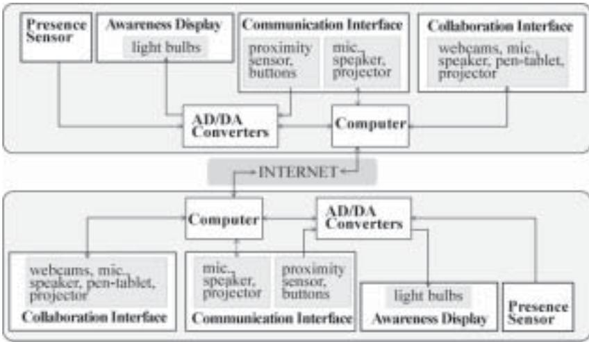
Figure 3. System architecture of our prototype system.
