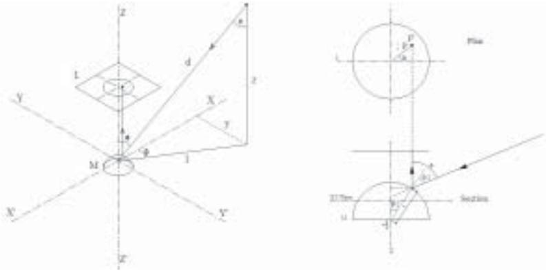
Figure 1. Coordinate system of spherical mirror projection.
