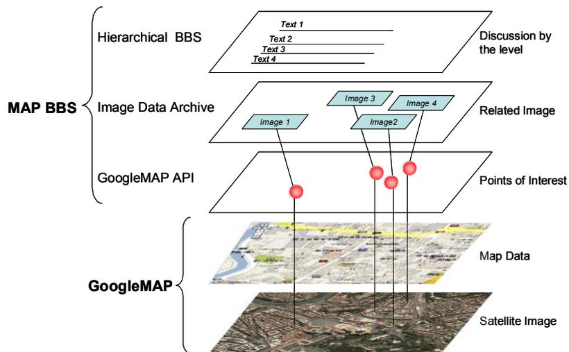
Figure2, Data structure of the map-based bulletin board system
