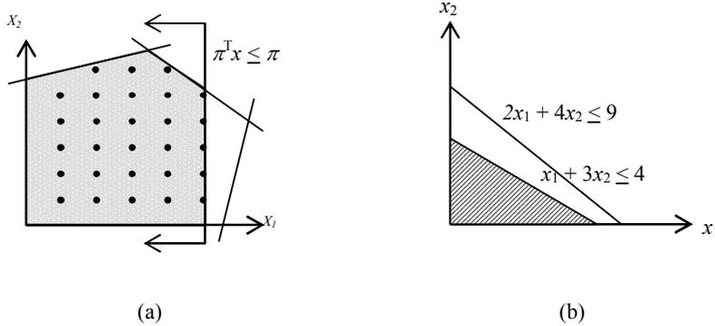
Figure 1. (a) the conceptual strong valid inequality cut  $\pi^T x \leq \pi$  is used to reduce the feasible region and (b) example, the strong valid inequality constraint  $x_1 + 3x_2 \leq 4$  dominates  $2x_1 + 4x_2 \leq 9$
