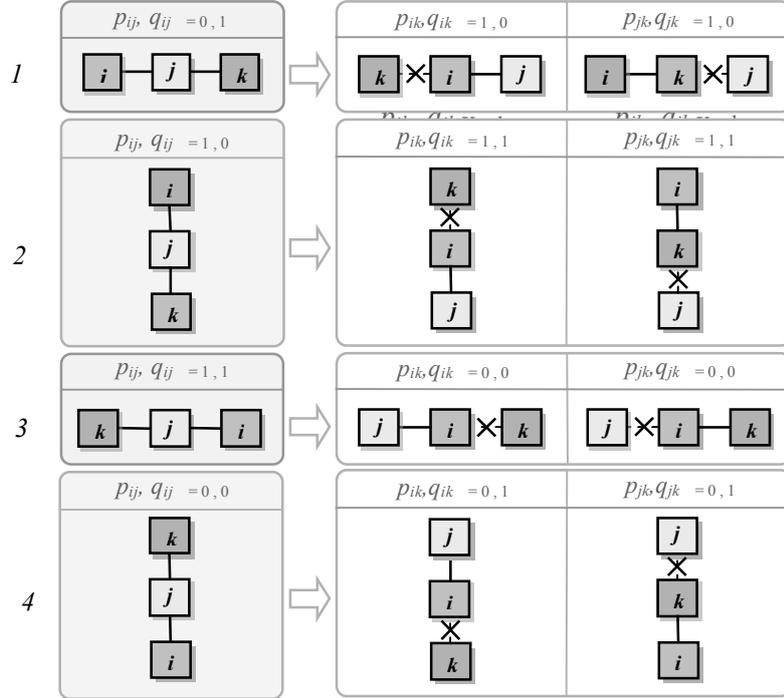
Figure 2. Show the concept of disconnected constraints, in case 1: If the connection of  $p_{ij}, q_{ij}$  is 0,0 then the connection of  $p_{ik}, q_{ik}$  and  $p_{jk}, q_{jk}$  can not be 1,0. Similarly, case 2,3 and 4 shows the disconnected configuration on the right side.
