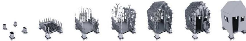
Figure 6: Construction sequence as simulated prior to construction.
