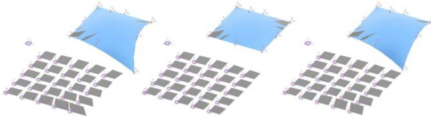
*Figure 3.* Being a parametric reproduction of the bspline surface, any adjustments on the geometry of the surface is passed its unfolded and subdivided version.
