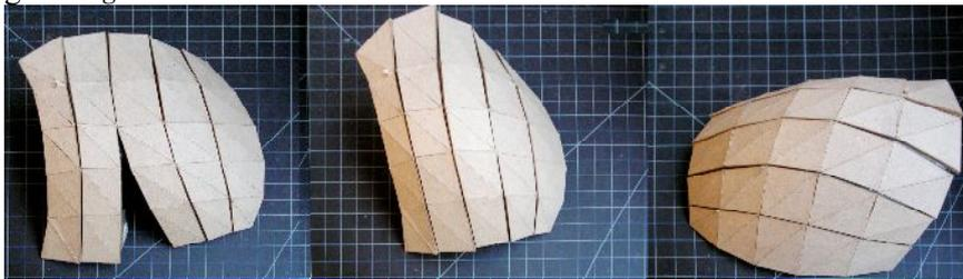
*Figure 4.* Assembling the pieces together to reconstruct the double curved structure.
