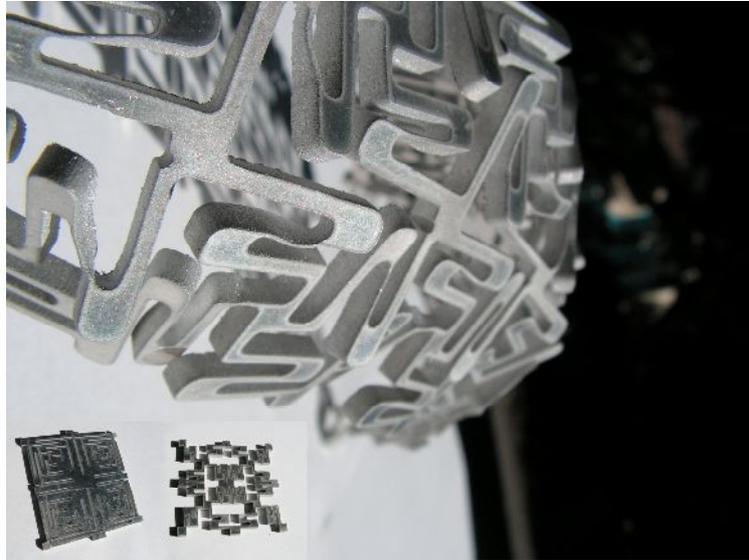
Figure 6. Pictures of flexure structures cut from 4 mm aluminum
