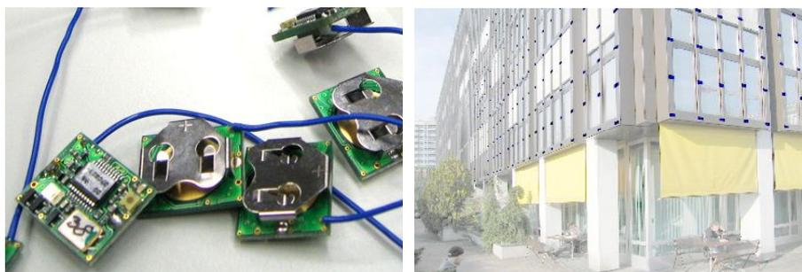
Figure 6. left: A 'particle computer' with integrated sensors and wireless connectivity. right: Illustration of the sensor network attached to a facade.
