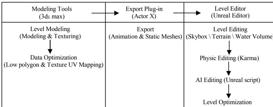
Figure 2: The working process of VR core engine.
