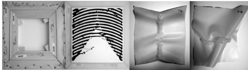
Figure 1: Resin impregnated latex-membrane experiments. Left: Rapid moulds designed for pre-stretching and impregnation. Right: Impregnation applied parallel and perpendicular to stretch to stretch.
