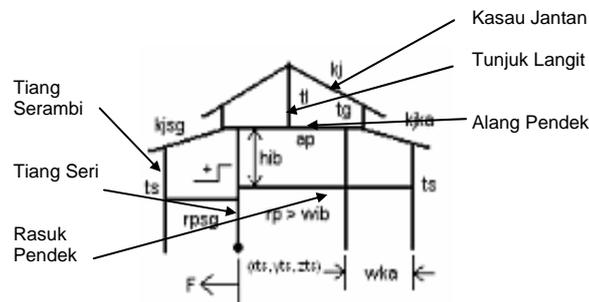
Figure 2. Primary construction elements of the TMH
