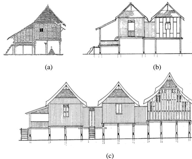
Figure 1. Examples of (a) 1-unit, (b) 2-unit and (c) 3-unit traditional Malay houses (adapted from Nasir, 1985).
